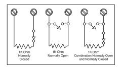
Figure 4: Protection Zone Wiring
