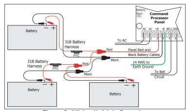
Figure 3: Wiring Multiple Batteries
