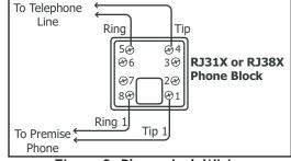
Figure 8: Phone Jack Wiring
