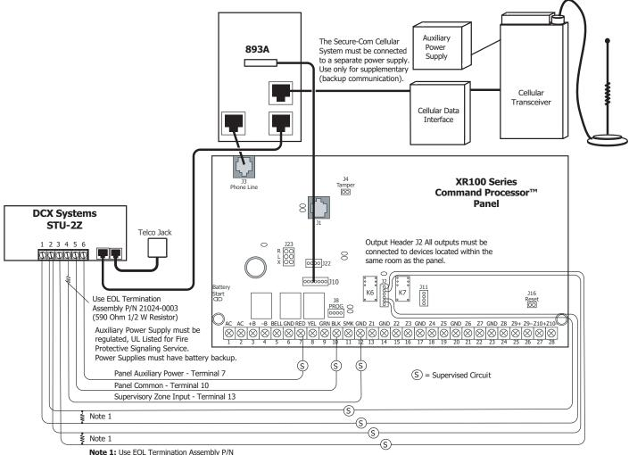
Note 1: Use EOL Termination Assembly P/I 21024-0001 (2.2k Ohm 1/2 W Resistor).
