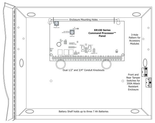
Figure 2: XR100 Series in Model 350 or 350A Enclosure
