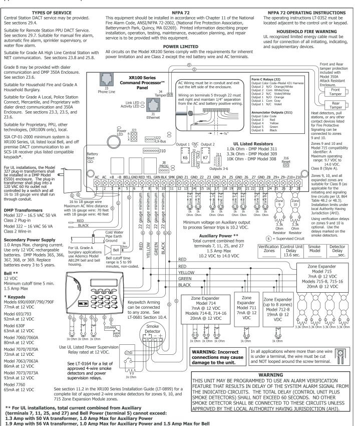
Figure 1: XR100 Series Wiring Diagram
